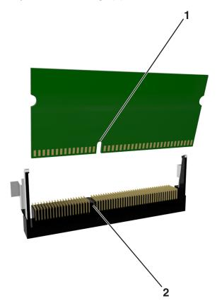
**4** Push the memory card straight into the connector and forward into the controller board wall until it *clicks* into place.
