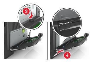
Run the ISP cable through the controller board shield.
