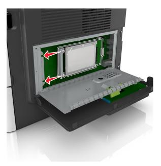
**c** Tighten the two screws.
