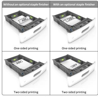
• Do not slide the paper into the tray. Load paper as shown in the illustration.
