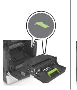
**Note:** Use the arrows on the side of the printer as a guide.
