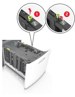
**b** If the A5 length guide is still attached to the length guide, then remove it from its place. If the A5 length guide is not attached, then proceed to step d.
