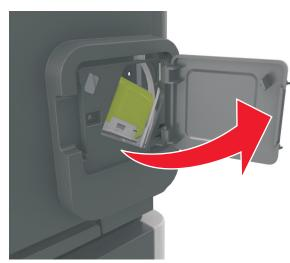
**3** Pull down the latch of the staple cartridge holder, and then pull the holder out of the printer.
