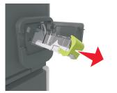
**4** Use the metal tab to lift the staple guard, and then remove any loose staples.
